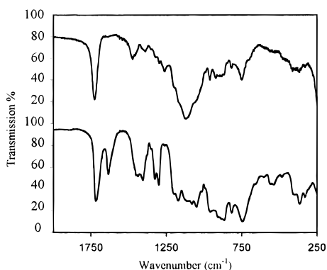
Figure 3. IR spectra of the sample obtained from the reaction of the polyanions \text{POM}_1 in the presence of the hydrosoluble initiator and in the absence of acrylamide (top) and of the starting solution (bottom).
